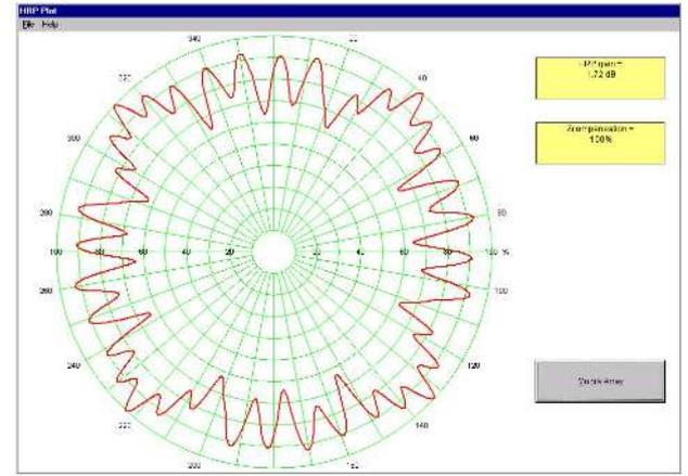
Skew Fire 4 Panels Radius 1465mm @ 740MHz
