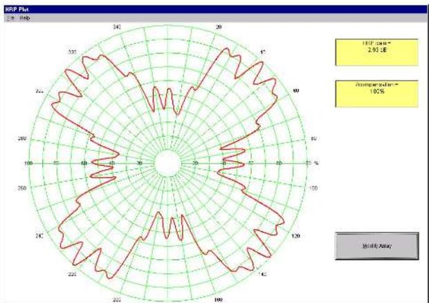
Skew Fire 4 Panels Radius 1465mm @ 680MHz
